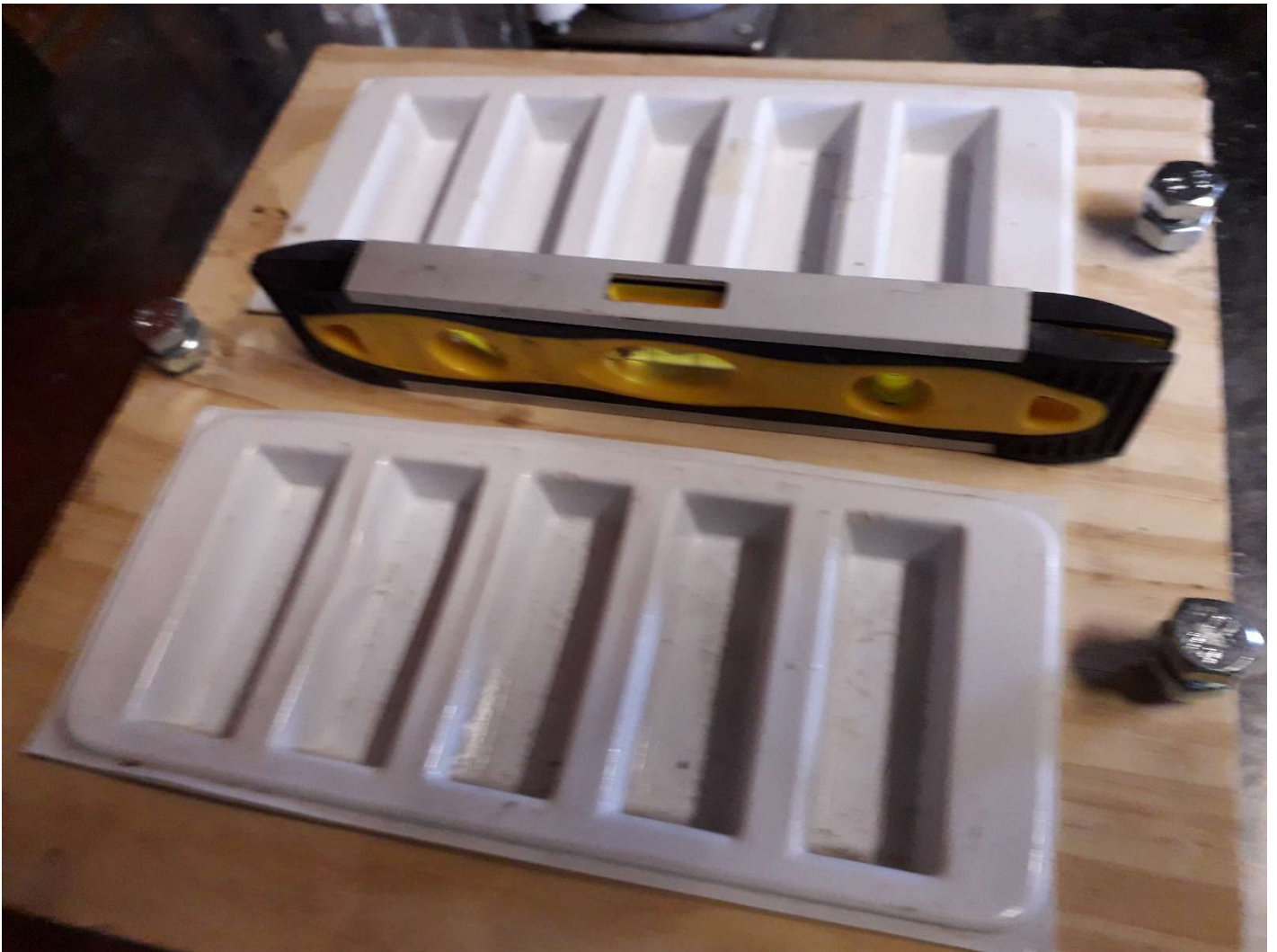
Plywood frame to hold wax moulds. Photo: John Goodwin.
